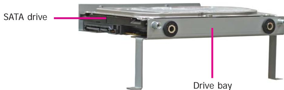
4. Use the provided mounting screws to secure the SATA drive onto the drive bay.
