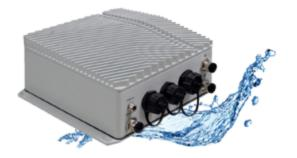
DFI's ECX700-AL Ruggedized Box PC is certified up to IP67 and supports industry-leading wide voltage and temperature to operate reliably outdoors. In addition, the system has waterproof connectors, further stopping any water from getting in. Due to the risks above to electronic circuitry from salt water, ECX700-AL's IP67 protection means that DFI's customers do not need to worry about electrical connections corroding or the overall system failing.
